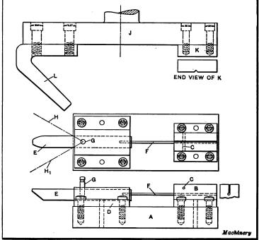
Fig. 14. Hinged Curling Die with Automatic Ejector
